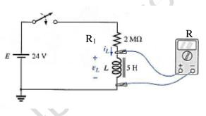
this EMF will flow the current in circuit available through the meter with resistance R. The magnetic field energy stored in the inductor during the growth of current through it is used to flow current through R and hence the energy and the current decrease with time.
