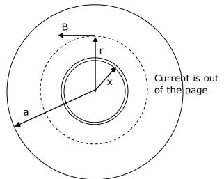
(a) For r = 0, B = 0. We have to consider the axis of the wire as loop and hence the area for the loop is zero giving the current in the loop zero and hence the magnetic field will be zero.
