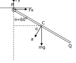
To find the acceleration of center of mass of the rod C, the easy way is to find the angular acceleration of the rod.
