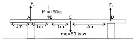
The weight of the plank mg is acting at its mid-point and the weight of the mass 150 kg is at 1m from the left support.
