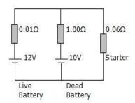
Let the current through the live battery is I, that through the starter be  $I_1$  and through dead battery is  $I_2$  then according to junction law the current through the live battery will be  $I = I_1 + I_2$ .
