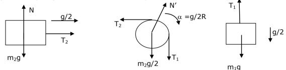
The vertical forces on the block of mass  $m_2$  are its weight  $m_2g$  and the normal reaction of horizontal surface N and will be balanced and the acceleration g/2 is provided by the tension  $T_2$  only hence according to the Newton's law of motion we have
