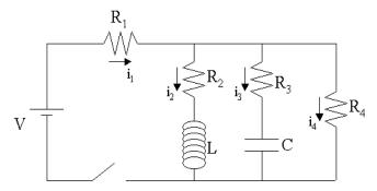
The switch has been open for a long time before it is closed at t = 0.
