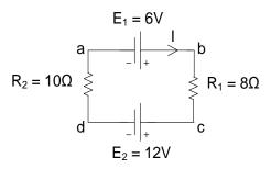
(a) Neglecting the internal resistances of the batteries, find the current in the circuit. Applying loop rule  $(\sum E = \sum R * I)$  for Clock wise direction as positive we can write
