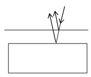
The additional path traveled by the light in the coating is 2\*t (t is thickness) and it is equivalent to the path difference  $2*t*\mu$  in air. Hence for minimum reflection we have
