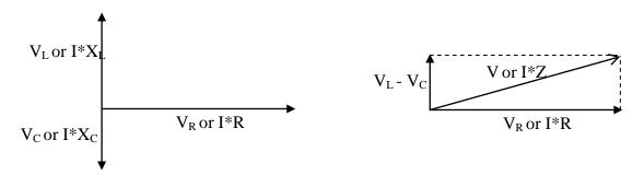
Hence the voltage amplitude across the whole circuit or of the supply generator is given by
