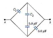
Looking minutely both terminals of  $C_1$  and 6.0  $\mu F$  capacitors are connected directly between the a and b. Similarly the series connection of 5.0  $\mu F$  and  $C_2$  is also connected directly to a and b. Thus the circuit is having  $C_1$ , 6.0  $\mu F$  capacitors and the series combination of 5.0  $\mu F$  and  $C_2$  are in parallel as in figure. The equivalent capacitance of the series combination of 5.0  $\mu F$  and  $C_2$  is equal to (units are in  $\mu F$ )
