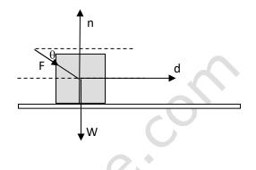
The weight W of the block is vertically downward means in negative y direction. The normal force n is acting on the block vertically up and in positive y direction.
