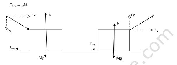
The normal reaction is the force equal and opposite to the resultant of the weight of the box Mg and the vertical component of the force applied.
