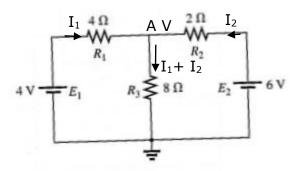
Let the current in the loops are  $I_1$  and  $I_2$  as in the figure and the potential at node A be V.
