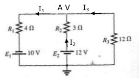
Let the current in the loops are  $I_1$  and  $I_2$  as in the figure and the potential at node A be V.
