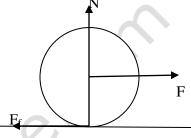
Here I is the moment of Inertia of the wheel about axis passing through center of mass of the wheel equal to  $\frac{1}{2}$  mR<sup>2</sup>.
