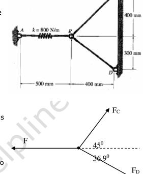
Now the geometry of the diagram shows that the force Fc is making an angle
